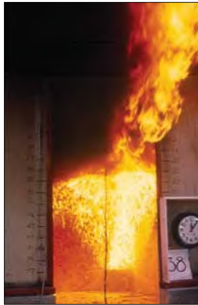
Figure 18-1. Flashover in standard room test.
